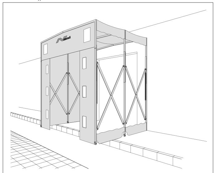
The Nani-Dockshelter type T-TAD protects the personnel and the commodity during the loading or unloading from influences of the weather. This type of door shelter is used with an external ramp, where the truck can be load or unload from the rear or also from the sides. The dock shelter consists of a front, a rear and, depending upon tunnel length, one or more middle frameworks, of stable, hot-dip galvanized steel sections.
