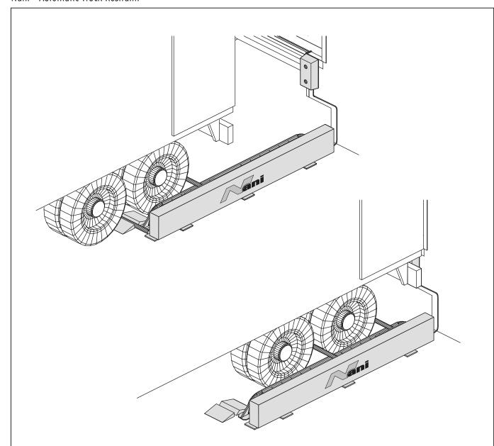
The automatic NANI-truck restraint is characterised by the fact, that it neither can be influenced by the truck-driver nor by the staff. That means that after the docking the truck can be moved neither intentional nor unintentional. When the truck is docking it drives with its rearmost wheel into the truck restraint and takes it in that way to the loading position. There comes it to an **automatic** locking of the truck restraint.
