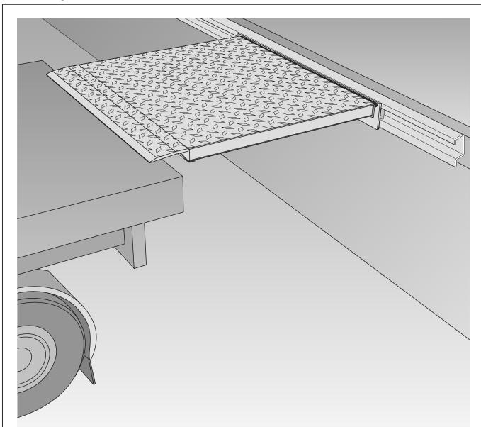
Spring counter balanced sliding loading bridge of high quality steel construction. The loading bridge is mounted on the edge of the loading dock. The edge of the dock must have a steel section incorporated to allow a special profile sliding track to be welded to it. This special profile is self cleaning.
